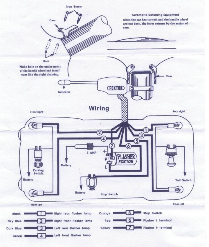
as each cord can be distinguishable by color, the wiring should be man: according to the above drawing \*\* Notice: Cam is not eed to install for non cancelling Switch.
