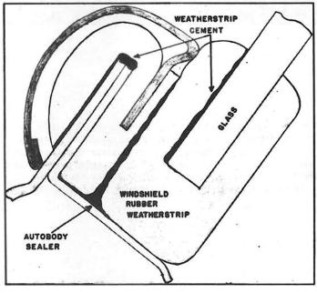
Before installation, the outer lip of the windshield rubber weatherstrip is cemented to the glass with "3-M Weatherstrip Cement", the complete assembly is then pressed firmly into the windshield opening. Note how the "Autobody Sealer" has spread out to affect a proper seal.
