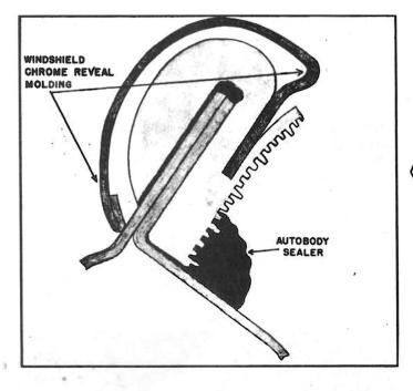
Next, the windshield chrome reveal molding is installed and then, prior to windshield installation, a heavy bead of "3-M Autobody Sealer" is applied clear around the opening at the area as shown.
