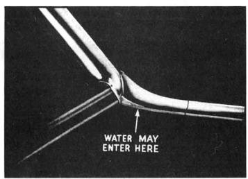
Clean all contacting surfaces with carbon-tetrachloride or clear gasoline (not ethyl) to remove dirt and old cement. After parts are thoroughly dry, apply a coating of "3-M Weatherstrip Cement" to contacting surfaces of cowl and gasket as shown by arrows 1 and 2 and fill chrome cap with "3-M Autobody Sealer" as indicated by arrow at 3. Permit cement to dry "tacky" (about ten minutes) before re-installing the molding. Wipe away all surplus cement sealer.
