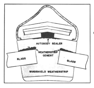
Center division section of windshield after windshield glass and weatherstrip has been installed. Note how "Autobody Sealer" has levelled off to affect a proper seal.
