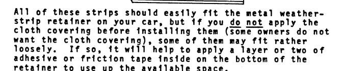
To determine right or left hand applications, usually a comparison with the old weatherstrip will tell you which side is which. Occasionally a small amount of additional end-trimming is necessary to get the kind of fit you want. Be very careful with this as the rubber strips should be long enough so that when the top is in place, the ends of the rubber strips meet each other.
